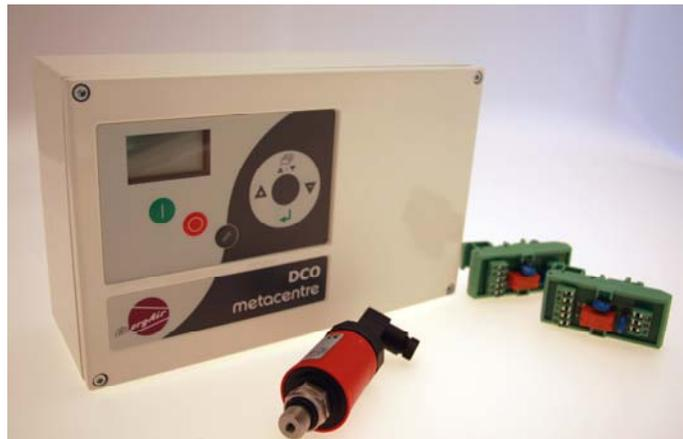
Metacentre™ DCO is a specialised supervisory control product designed to provide energy efficient optimised narrow pressure and priority management control of up to 4 air / gas compressors operating in a common compressed air / gas system. Each DCO kit is provided with a quantity of compressor interface PCB's (mi-PCB) and a 4-20mA / 0-16bar pressure sensor.
