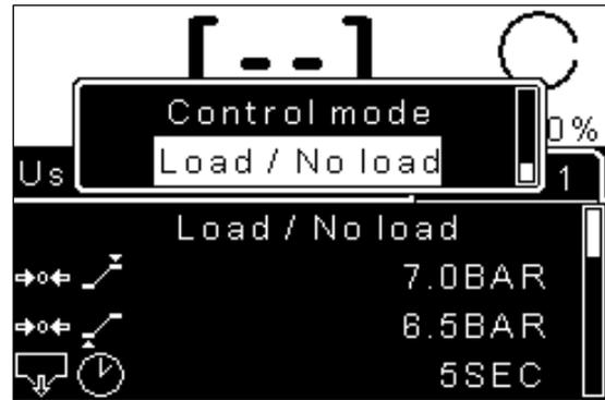
An edit menu popup window will appear. Use the Up and Down keys to select an available option. Press and hold the Up or Down key to increase the speed at which a selectable value is reached. Press the enter key to confirm a selection or use the clear key to exit without making a new selection.
