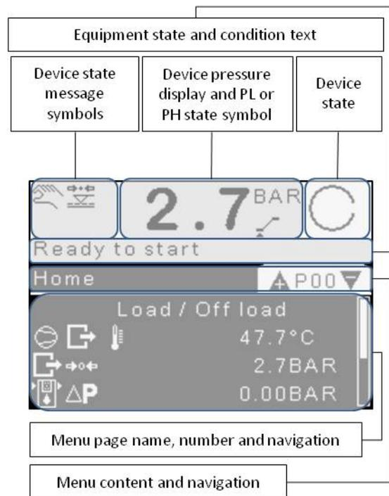
After a period of non-use the graphic display light level will reduce until a key is pressed.
