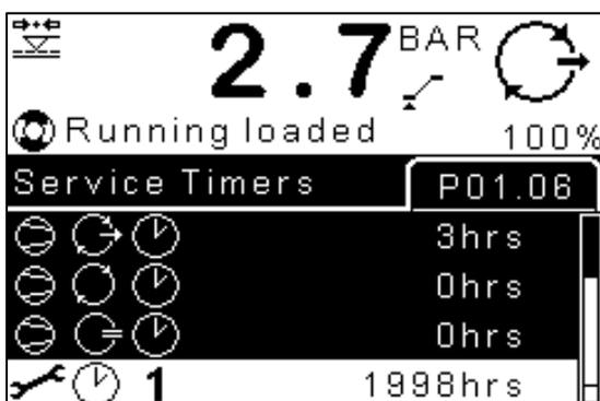
To edit an accessible and editable menu item, navigate to it and press the enter key.
