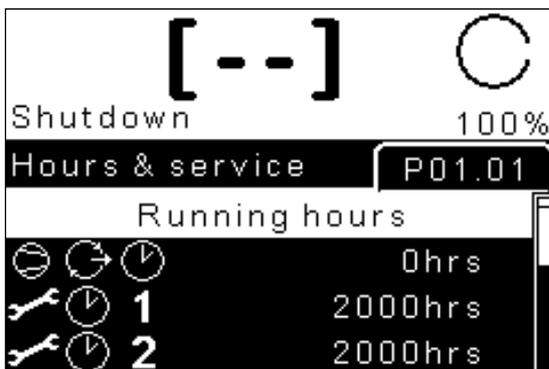
Entering the menu content area navigates to the first item of the menu. Use the Up and Down keys to navigate between menu content items. Menu content items are vertically assembled and in a continuous loop. For example, below indicates the user has navigated to P01 menu item 06
