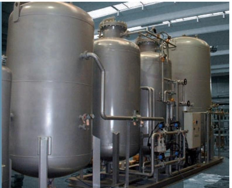
A nitrogen generator plant consists in a train with different components, to obtain nitrogen from compressed air.
