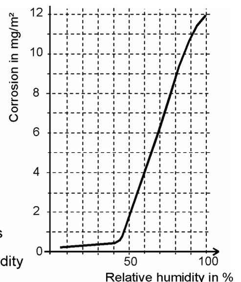
Corrosion as a function of relative humidity
