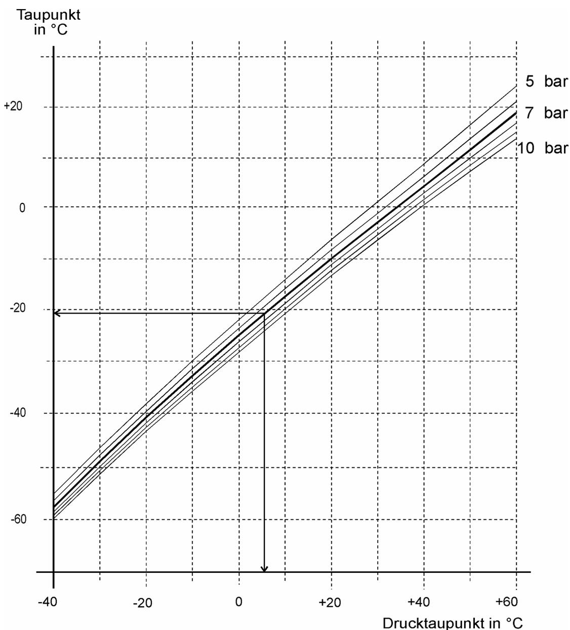
**Пример:** PDP =  $+5^\circ\text{C}$   $\rightarrow$  DP =  $-20^\circ\text{C}$
