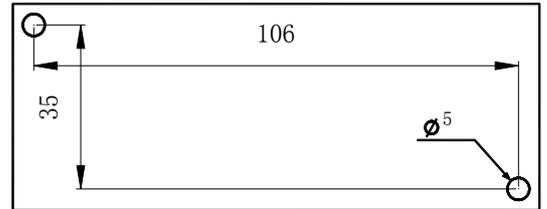
Figure 4.1.2. Installation dimension of CT 1
