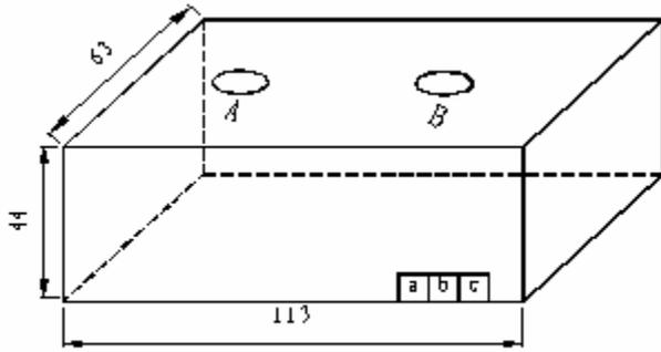
Figure 4.1.1. Structure dimensions of CT1 (φ36 through hole)
