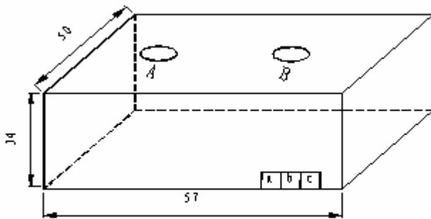
Figure 4.1.3. Structure dimensions of CT2 (φ10 through hole)
