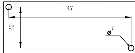
Figure 4.1.4. Installation dimensions of CT2
