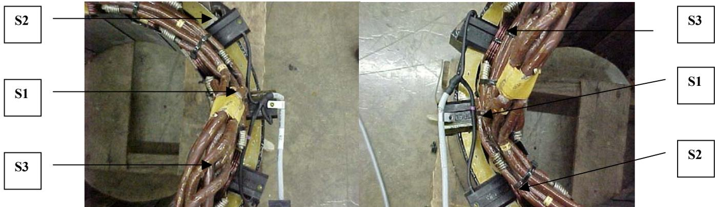
**When the new hall effect sensor kits are installed, the sensors will need to be placed in the order that is shown in the illustration above. The ground was previously mounted to the S3 sensor.**
