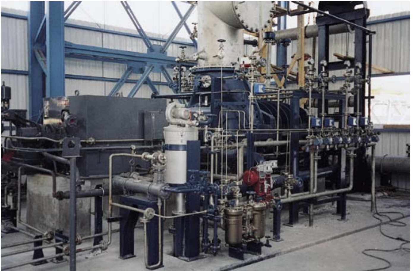
Aerzen screw compressor unit VRa 836 L for the compression of lime kiln gas
