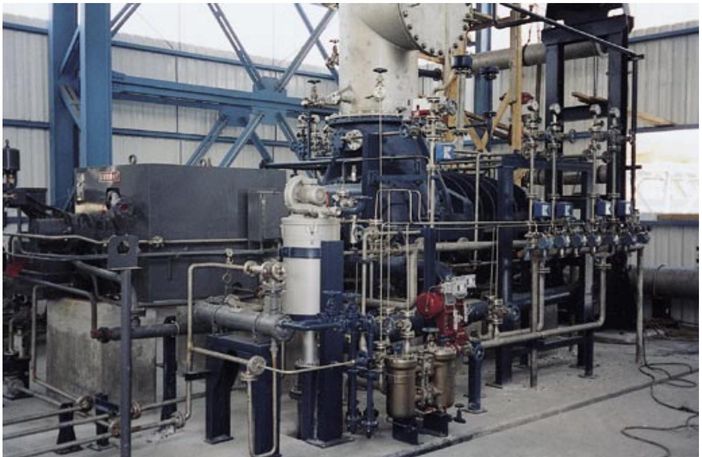
VRO 836 L for compression of lime kiln gas
