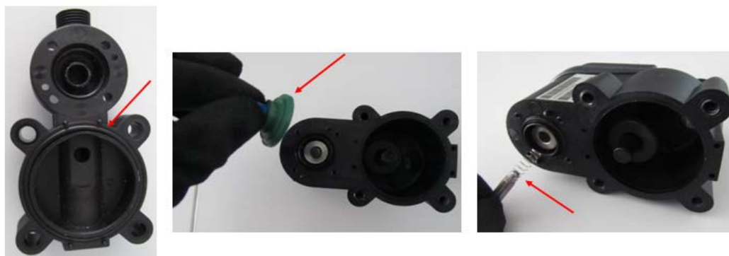
Fig. 4.a ED12 drain disassembly
