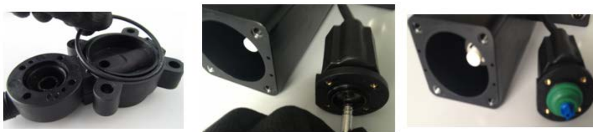
Fig. 5.b LD drain reassembly
