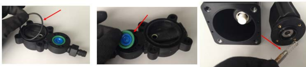
Fig. 4.b LD drain disassembly
